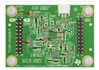
J8 is the enable pin for the 3.3V Regulator. Remove this jumper and the 3.3V Regulator will not start up.
