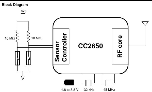
Figure 7. System Block Diagram
