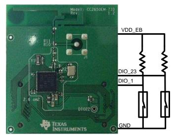
Figure 9. Circuit Connection to CC2650EM-71D
