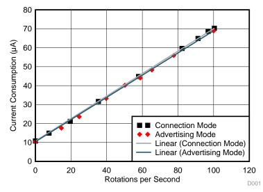
Figure 12. Test Results of Advertising Mode and Connected Mode
