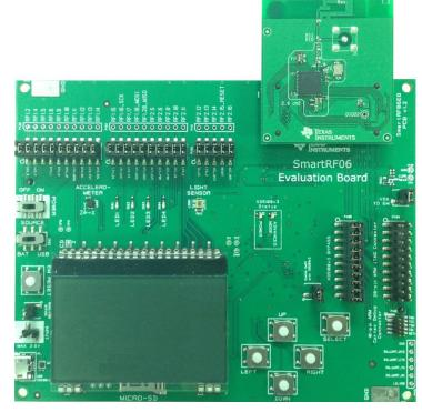
Figure 8. CC2650EM-71D Plugged Onto SmartRF06 Evaluation Board
