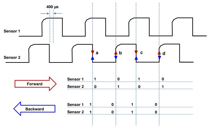
Figure 6. Direction Detection With Two Sensors
