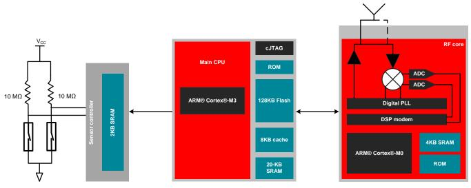
Figure 1. Signal Flow Among Sensor Controller, Main CPU, and RF Core of CC2650
