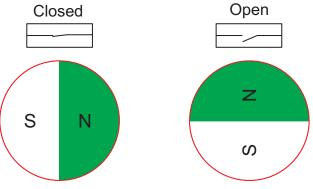
Figure 4. Reed Switch Over a Magnetic Rotor
