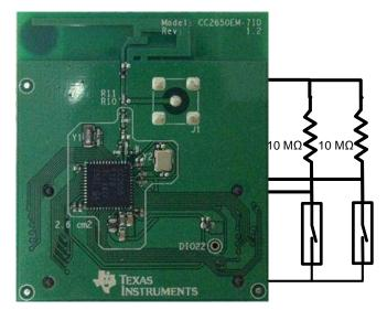
Figure 3. Single Chip on CC2650EM-71D
