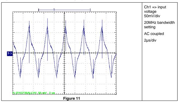
The input ripple voltage is shown in **Error! Reference source not found.** The image was taken with 0.5A load 12V at the input. The waveforms were captured timely separate.
