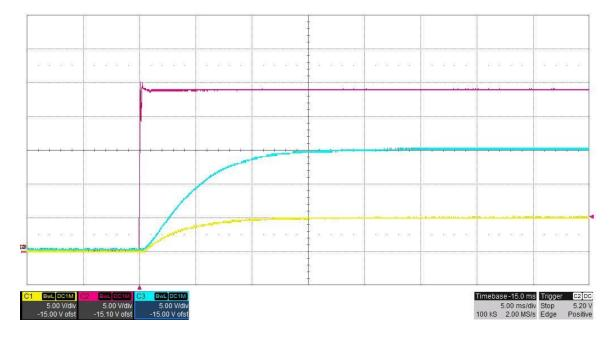
The photo below shows the **15V#2 and 5V#2** output voltage startup waveform, measured at TP16 and TP20, after the input voltage is applied. Vin = 24V, Iout = **0.15A**. (5V/DIV, 5mS/DIV)
