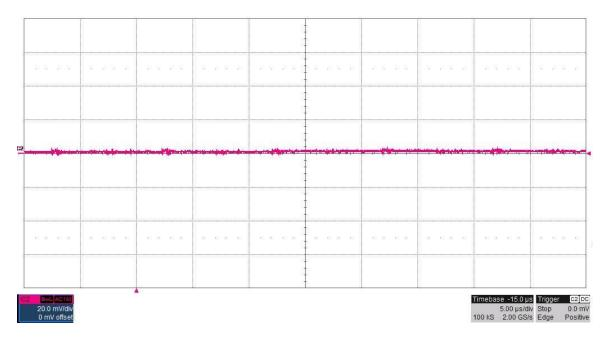
The output ripple voltage is shown in the figure below. The image was taken with the 15V#1 output loaded to 0.15A and the input voltage set to 26.4V. (20mV/DIV, 5uS/DIV)
