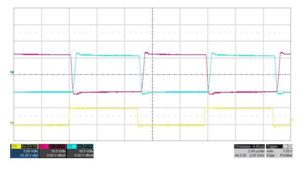
The photo below shows the switch node voltages of 15V#2 and 5V#2, measured at TP18 and TP25 and the PHASE clock signal. Vin = 21.6V, Iout = 0.15A. (PHASE is 5V/DIV, 10V/DIV, 2uS/DIV)
