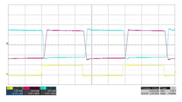
The photo below shows the switch node voltages of 15V#1 and 5V#1, measured at TP4 and TP12 and the PHASE clock signal. Vin = 26.4V, Iout = 0.15A. (PHASE is 5V/DIV, 10V/DIV, 2uS/DIV)
