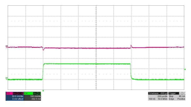
The photo below shows the **15V#1** output voltage (ac coupled) when the load current is stepped between 0A and 0.15A. Vin = 24V. (50mV/DIV, 100mA/DIV, 200uS/DIV)
