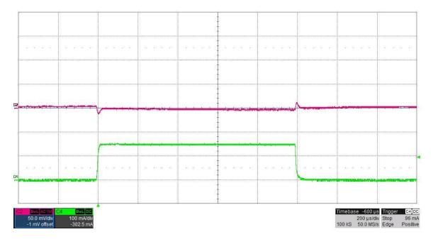
The photo below shows the **15V#2** output voltage (ac coupled) when the load current is stepped between 0A and 0.15A. Vin = 24V. (50mV/DIV, 100mA/DIV, 200uS/DIV)
