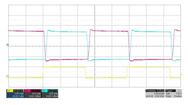
The photo below shows the switch node voltages of 15V#2 and 5V#2, measured at TP18 and TP25 and the PHASE clock signal. Vin = 26.4V, Iout = 0.15A. (PHASE is 5V/DIV, 10V/DIV, 2uS/DIV)
