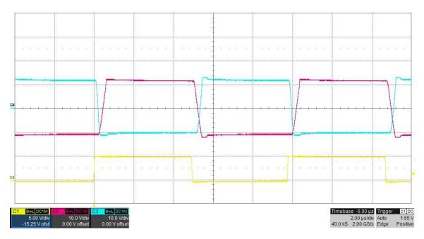
The photo below shows the switch node voltages of 15V#1 and 5V#1, measured at TP4 and TP12 and the PHASE clock signal. Vin = 21.6V, Iout = 0.15A. (PHASE is 5V/DIV, 10V/DIV, 2uS/DIV)
