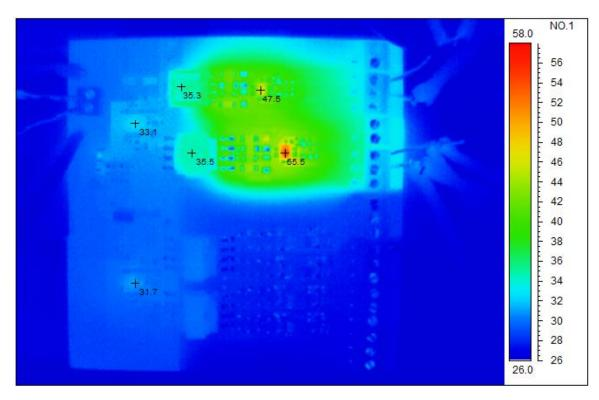
The thermal image below shows the temperature rise with 24Vin and 15V#2 @ 0.15A and 5V#2 @ 0.15A, with no airflow. All other outputs are unloaded.
