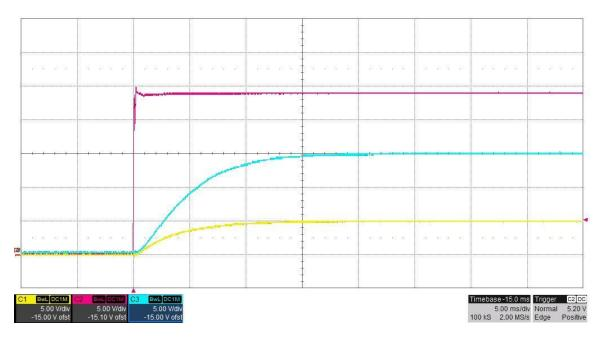
The photo below shows the **15V#1 and 5V#1** output voltage startup waveform, measured at TP2 and TP11, after the input voltage is applied. Vin = 24V, Iout = **0.15A**. (5V/DIV, 5mS/DIV)
