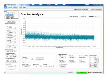
Figure 40. OPA625 GND Rail Full Swing Result
