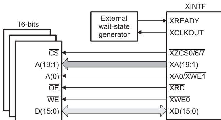
When an XINTF zone is configured for 32-bit mode (XTIMINGx[XSIZE] = 1), the XA0/XWE1 signal is the active low write strobe  $\overline{XWE1}$ .  $\overline{XWE1}$  is used, along with  $\overline{XWE0}$  for 32-bit bus operation as shown in Figure 5.
