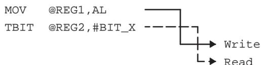
The 28x CPU automatically protects writes followed by reads to the same memory location. The protection mechanism described above is for cases where the address is not the same, but within a given region of protected memory. In this case, the order of execution is preserved by the CPU automatically inserting enough NOP cycles for the write to complete before the read occurs.
