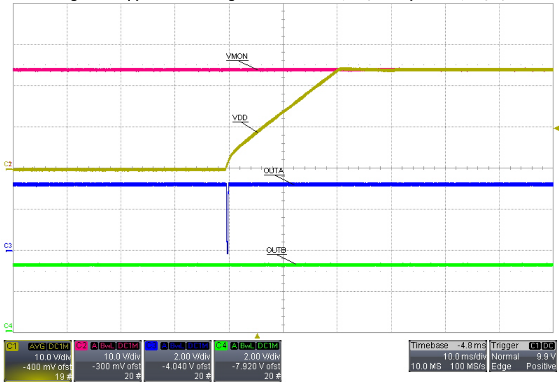
Figure 7: Startup with V_{DD} , V_{MON} Independent, V_{PULLUP} = 3.3
