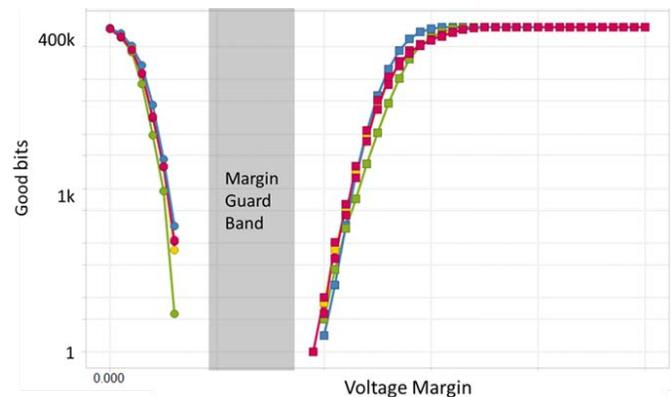
Fig. 4. 1T-1C bit distributions of voltage margin across entire FRAM array for Pre- and Post- TID exposure for all devices exposed from 75krad(Si) to 300krad(Si). The “1”s distribution is on the right and the “0”s is on the left. Reliability mechanisms tend to reduce “1”s margin (shifting the right-hand curve to lower margins)
