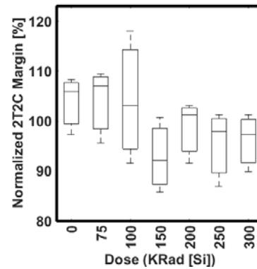
Fig. 3. 2T-2C Normalized margin change over different test insertions and TID exposures. The average normalized margin varies less than 10% over all TID exposure levels with worst-case observed margin of ~ 85%. The FRAM can read data down to a normalized margin of ~ 20%.
