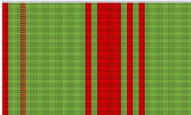
Fig. 10 Bit map showing block level failures seen due to redundant SRAM upsets during SEU testing of the FEDC FRAM. The bitmap shows the boundary fails (red stripes) on 128 bit intervals - implying that SEU in the RSRAM are the root cause. No SEFIs were observed in the FEHT FRAM.
