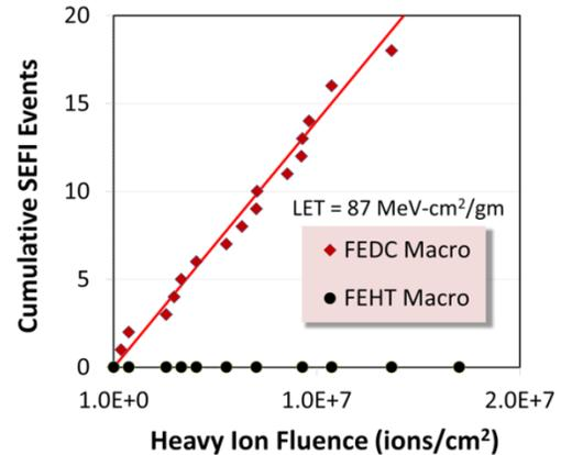
Fig. 11. Plot of observed RSRAM-induced SEFI events (block failures) as a function of heavy ion fluence (LET=87 MeV-cm<sup>2</sup>/mg). Note that while FEDC FRAM exhibited many SEFI events, NO SEFI events were observed in the FEHT FRAM with hardened RSRAM block.
