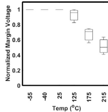
Fig. 6. Normalized Margin % Change vs. Temperature. Decrease in the spontaneous polarization is expected as temperature is increased in ferroelectric materials due to the thermal depolarization effect [2].
