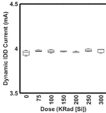
Fig. 5. Dynamic Write/Read current vs. dose. The dynamic W/R current was essentially independent of the TID exposure levels in this FRAM.
