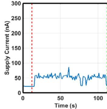
Fig. 9. Typical power supply curve seen during SEL testing. The red/green dotted lines represent where the beam was turned on/off respectively. Supply current increases during irradiation because of ion generated SCR charge. If SEL occurs, a large jump in current is expected as the parasitic SCR is established. No SEL events were observed in any of the FEDC or FEHT FRAM tests.
