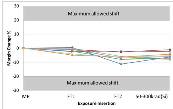
Fig. 2. 1T-1C Margin change percent over different test insertions and TID exposures. Each line is an individual device at all steps through the screening process. It should be noted that the maximum allowed shift is not a functional failure. There is still much more margin in the design.
