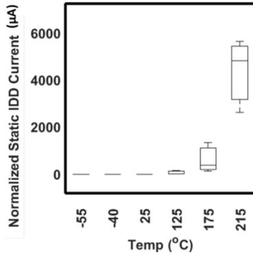
Fig. 8. Normalized static supply current vs. temperature. Dominated by junction leakage, the current rises exponentially with increasing temperature.
