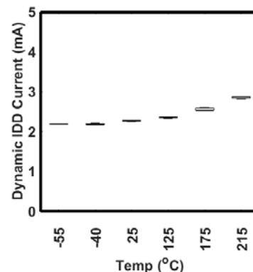
Fig. 7. Normalized dynamic supply current during active write/read vs. temperature. This is expected since dynamic current is dominated by the FeCap switching current which is not a strong function of temperature.
