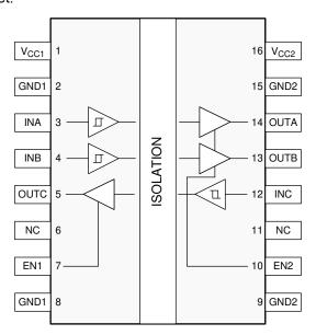
Figure 4-1. Pin Diagram (16-DW) Package
