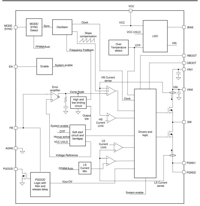
Figure 1-2. Functional Block Diagram: LMQ62440-Q1
