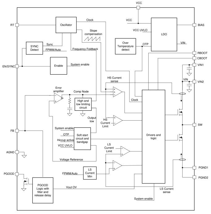
Figure 1-1. Functional Block Diagram: LMQ61460, LMQ61460-Q1
