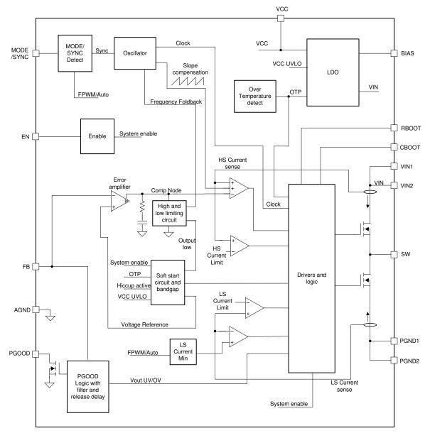
Figure 1-1. Functional Block Diagram
