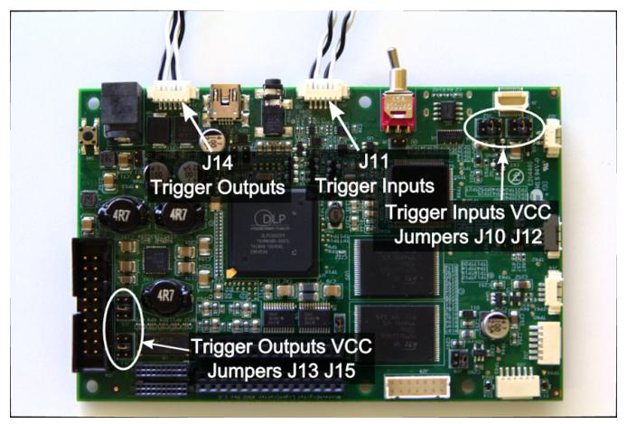
Figure 1. DLP LightCrafter 4500 Controller Board
