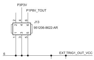
J13: The desired voltage level for trigger out 1 is selected by the insertion of a jumper between the appropriate pair of pins.
