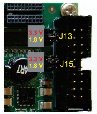
In this example, the jumpers are installed for 3.3 V.
