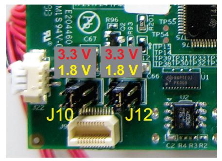
Example, the jumpers are installed for 3.3 V.
