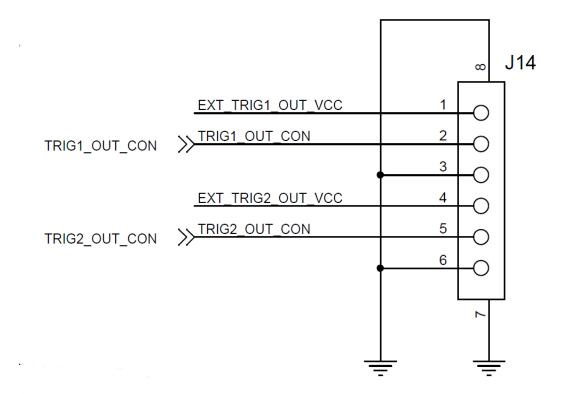
Figure 2. Schematic of J14 – Trigger Out 1 and 2
