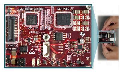
Figure 4-2. DLP .2 nHD (DLP2000) Chipset Evaluation Module (EVM) Electronics
