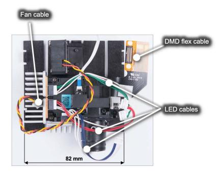
Figure 4-4. DLP Pico .23 1080p (DLP230NP) Display Optical Engine
