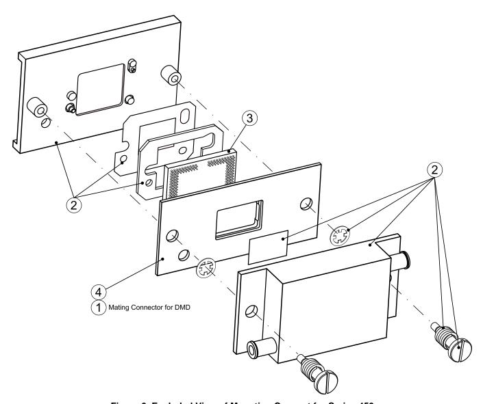
Figure 6. Exploded View of Mounting Concept for Series-450
