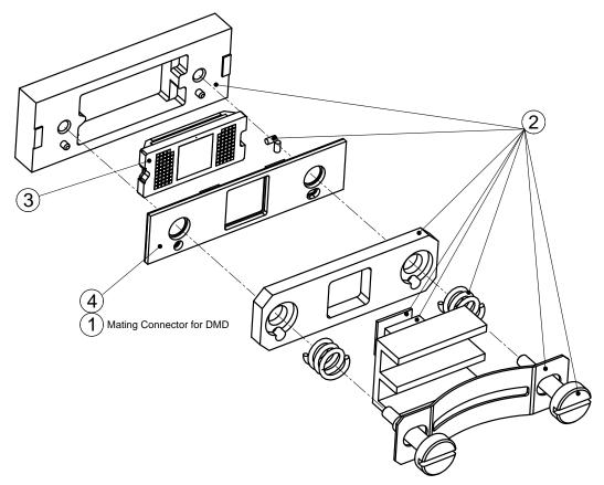
Figure 4. Exploded View of Mounting Concept for Series-310
