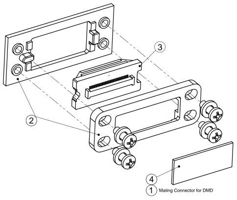
Figure 2. Exploded View of Mounting Concept for Series-220
