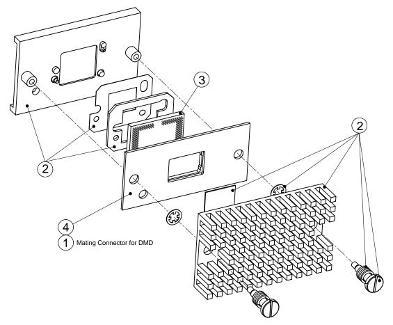
Figure 5. Exploded View of Mounting Concept for Series-450
