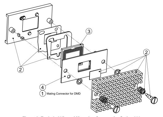
Figure 8. Exploded View of Mounting Concept for Series-600
