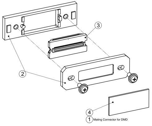
Figure 3. Exploded View of Mounting Concept for Series-241
