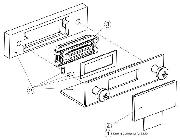
Figure 1. Exploded View of Mounting Concept for Series-244
