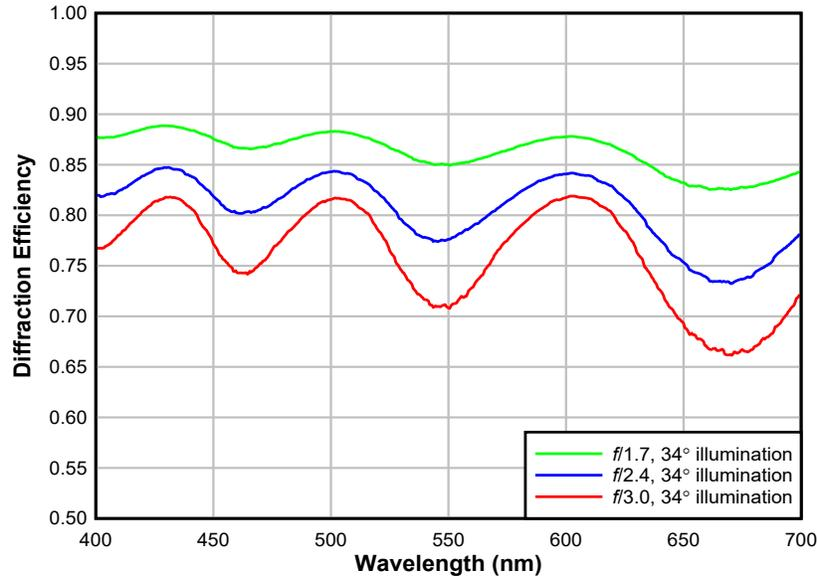
**Figure 4-7. 5.4 μm Pitch DMD Mirror Calculated Diffraction Efficiency (matched illumination and projection  $f$ -numbers)**
