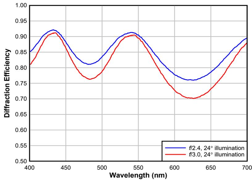
Figure 4-6. 7.56  $\mu\text{m}$  Pitch DMD Mirror Calculated Diffraction Efficiency (matched illumination and projection  $f$ -numbers)
