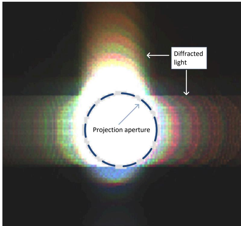
Figure 4-1. Simulated 5.4 μm Pitch DMD Far Field Radiance Image; Dashed Circle Shows Outline of Projection Lens Aperture Edge
