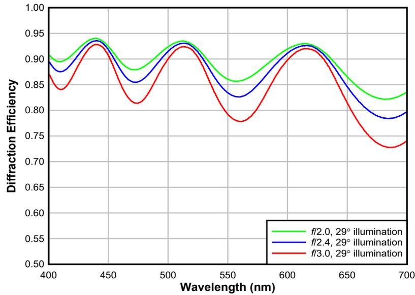
Figure 4-5. 9.0  $\mu\text{m}$  Pitch DMD Mirror Calculated Diffraction Efficiency (matched illumination and projection  $f$ -numbers)
