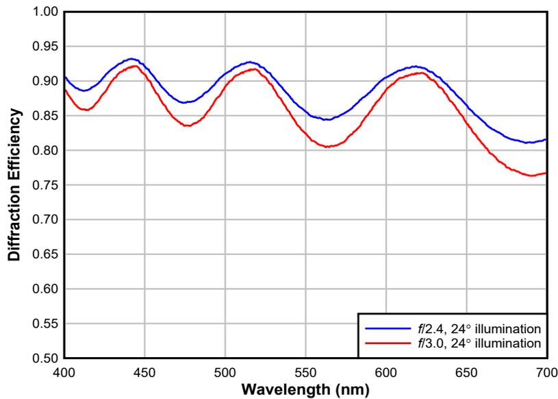
Figure 4-4. 10.8  $\mu\text{m}$  Pitch DMD Mirror Calculated Diffraction Efficiency (matched illumination and projection  $f$ -numbers)
