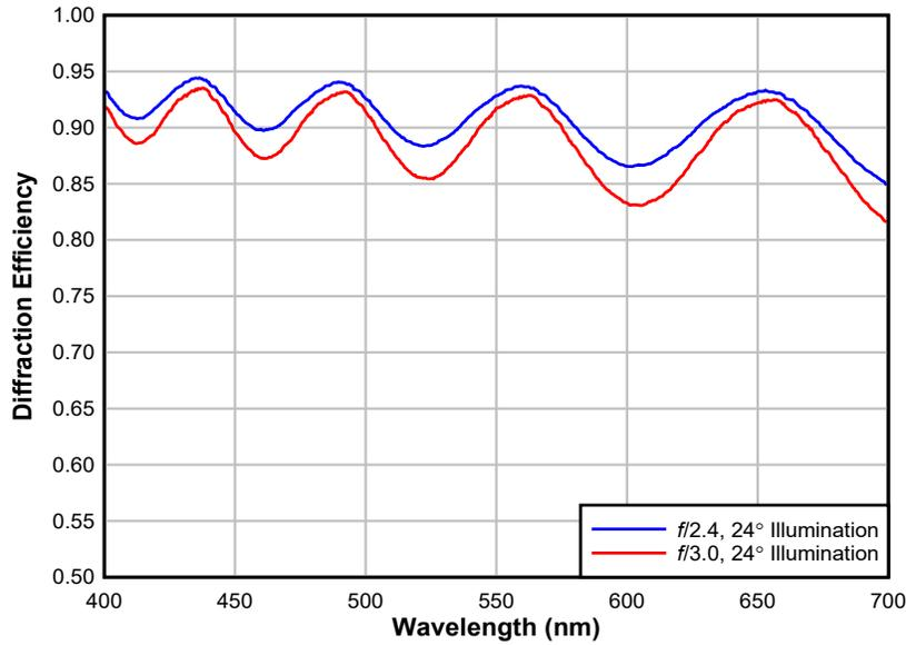
Figure 4-3. 13.68  $\mu\text{m}$  Pitch DMD Mirror Calculated Diffraction Efficiency (matched illumination and projection  $f$ -numbers)
