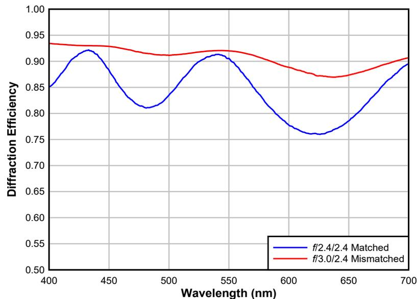
**Figure 4-8. 7.56 μm Pitch DMD Mirror Calculated Diffraction Efficiency With Matched and Mismatched  $f$ -numbers**
