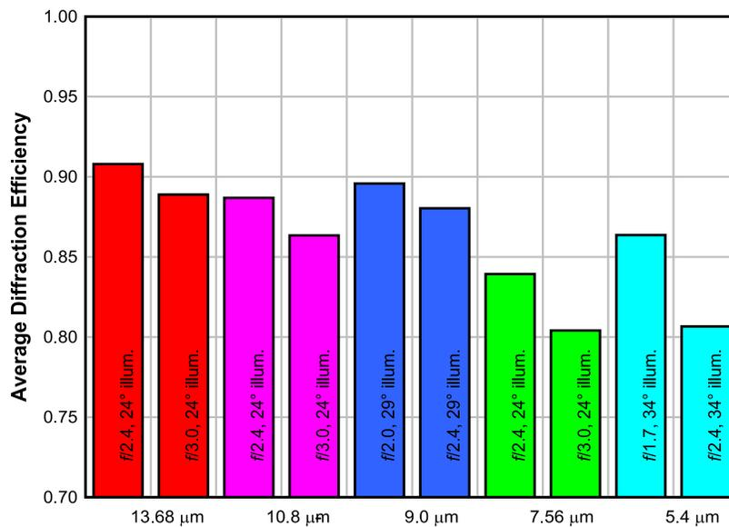
Figure 4-2. Summary of Calculated Average Photopic Diffraction Efficiencies for Different Pixel Sizes (420 nm–680 nm wavelength)
