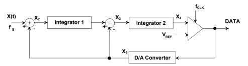
Figure 4. Block Diagram of the 2nd-Order Modulator
