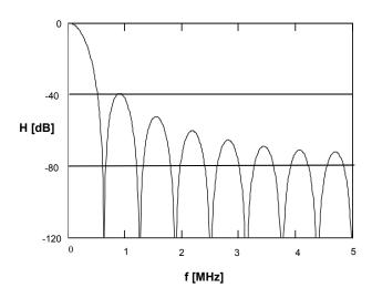
Figure 10. Frequency Response of the Sinc<sup>3</sup> Filter with M = 16
