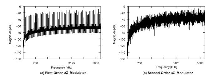
Figure 5. 1st and 2nd Order  $\Delta\Sigma$  Modulator Modulation Noise
