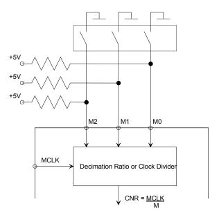
Figure 14. Clock Divider Inputs
