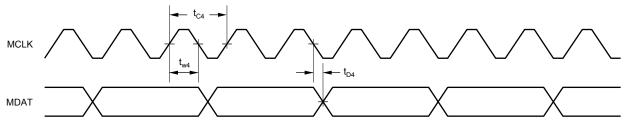
Figure 2. ADS1202 Output Read Operation
