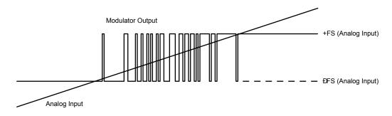
Figure 3. Analog Input versus Modulator Output of the ADS1202
