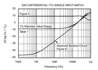
Figure 13. Difference in Input Impedances over Frequency
