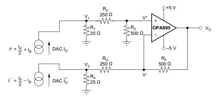
Figure 5. Initial Design Using the OPA695
