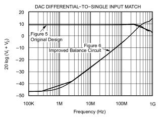
Figure 8. Simulated Difference in the Input Voltage
