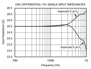
Figure 10. Improved Design Impedance at  $V_1$  and  $V_2$
