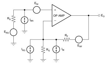
Figure 11. Output Noise Analysis Circuit
