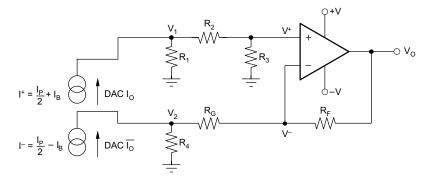
Figure 3. Analysis Circuit for Single Amplifier (Differential to Single-Ended Conversion)
