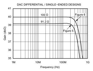
Figure 7. Simulated Frequency Response Comparison
