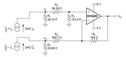
Figure 6. Improved Design Using the OPA695
