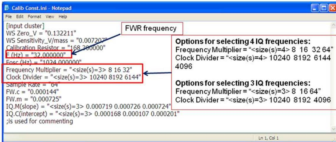
Figure 4. AFE4300 GUI Calib Const.ini Setting
