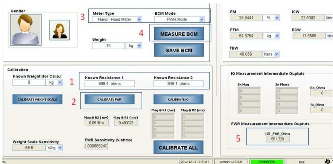
Figure 9. Impedance Measurement in FWR Mode with the AFE4300 GUI
