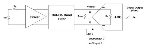
Figure 2. ADC Input Impedance and Transfer Function
