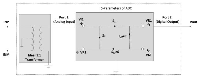
Figure 10. Ideal 1:1 Transformer in Front of S-Parameter ADC Model
