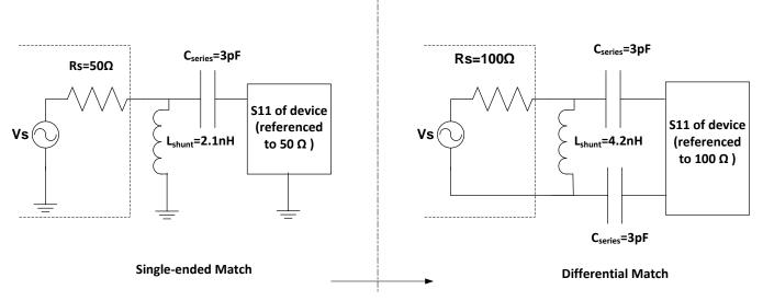
Figure 14. Single-Ended and Equivalent Differential Matching Network
