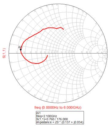
Figure 8. Differential S11 on Smith Chart ( $Z_0 = 100 \Omega$ )
