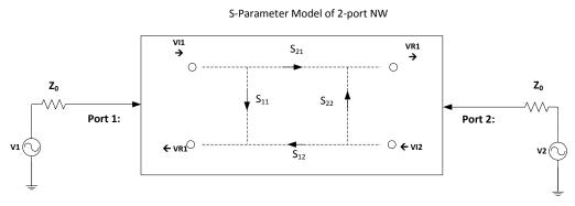
Figure 5. S-Parameter Model for a 2-Port Device
