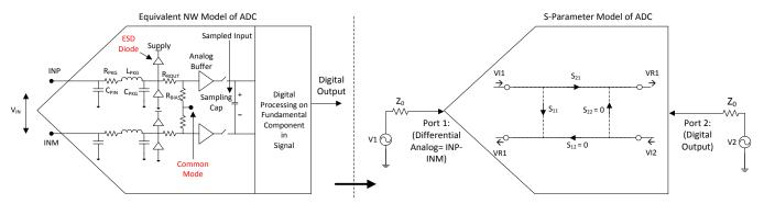
Figure 7. Equivalent NW Model and S-Parameter Model for ADC With S12 and S22 Chosen as 0
