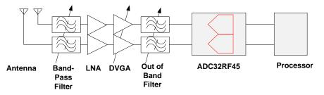
Figure 1. RF-Sampling ADC in RX Signal Chain
