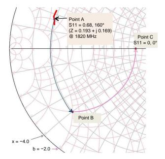
Figure 13. Finding Matching Network Using Smith Chart at 1.82 GHz
