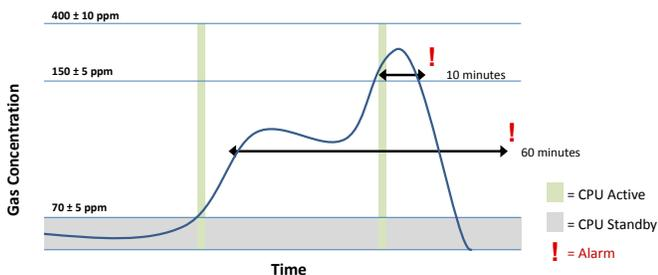
**Figure 4. CPU Activity Using the ADS7142**
