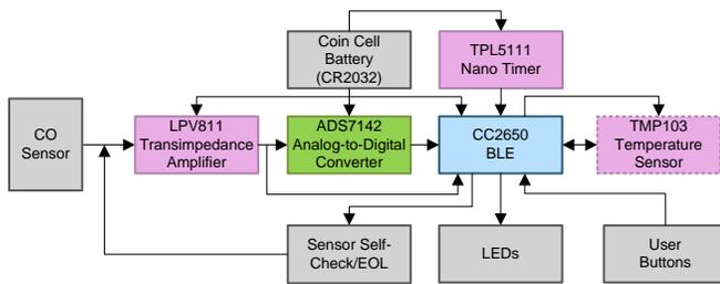
**Figure 3. Gas Sensor Node Using ADS7142**
