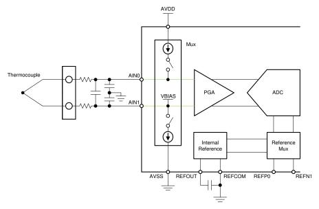
Figure 2-4. Thermocouple Measurement Circuit With VBIAS for Sensor Biasing and BOCS
