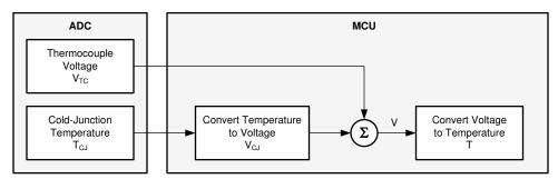
Figure 1-7. Thermocouple and Cold-Junction Measurement Conversion to Temperature
