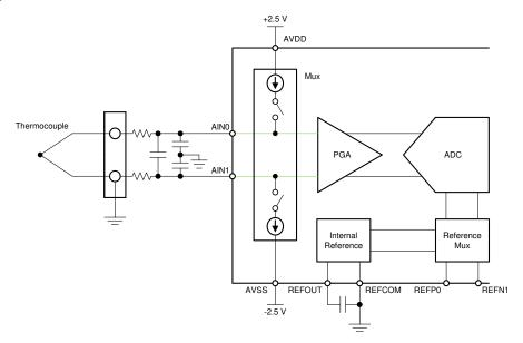
Figure 2-7. Thermocouple Measurement Circuit With Bipolar Supplies and Ground Biasing
