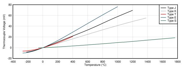
Figure 1-2. Thermocouple Responses
