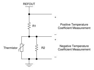
Figure 2-11. Linearization of Thermistor With Parallel Resistor and Voltage Divider
