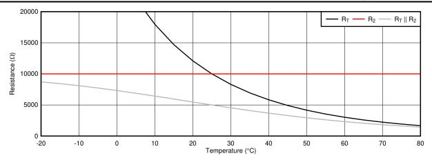
Figure 2-10. Thermistor and Linearization Responses Over Temperature
