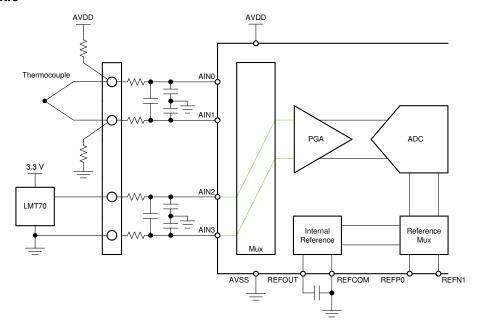
Figure 2-13. Thermocouple Measurement Circuit With Temperature Sensor Cold-Junction Compensation
