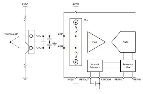
Figure 2-2. Thermocouple Measurement Circuit With Biasing Resistors Attached to the Negative Lead
