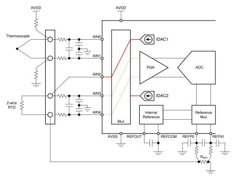
Figure 2-8. Thermocouple Measurement Circuit With Two-Wire RTD Cold-Junction Compensation
