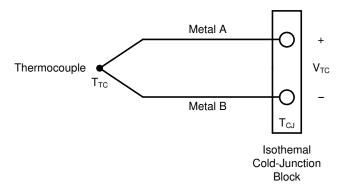
Figure 1-1. Thermocouple Voltage
