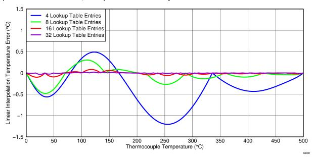
Figure 1-8. Comparison of Interpolation Errors Using Various Lookup Tables
