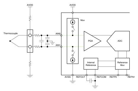
Figure 2-1. Thermocouple Measurement Circuit With Pullup and Pulldown Resistors
