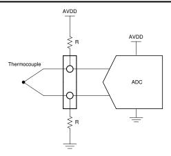
Figure 1-5. Resistor Biasing of a Thermocouple
