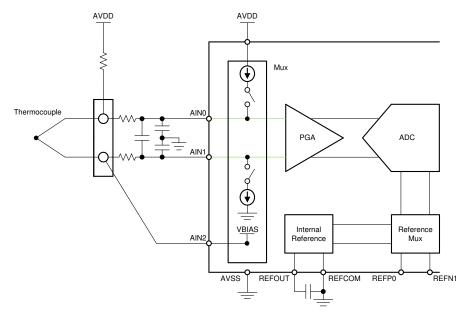
Figure 2-3. Thermocouple Measurement Circuit Using VBIAS For Sensor Biasing and Pullup Resistor
