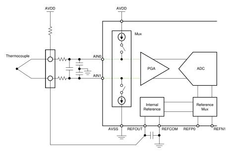
Figure 2-5. Thermocouple Measurement Circuit With REFOUT Biasing and Pullup Resistor
