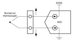
Figure 1-10. Burn-out Detection Using BOCS
