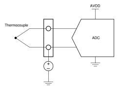
Figure 1-6. Voltage Biasing of a Thermocouple
