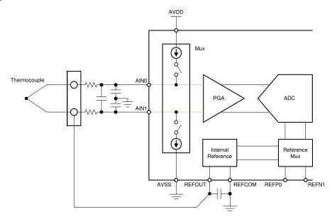
Figure 2-6. Thermocouple Measurement Circuit With REFOUT Biasing and BOCS
