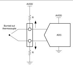
Figure 1-9. Burn-out Detection Using Resistor Biasing
