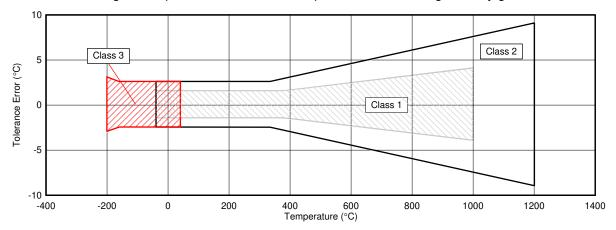
Figure 1-4. Type-K IEC-EN 60584-2 Tolerance Class Errors
