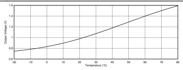
Figure 2-12. Linearized Output of Thermistor Circuit
