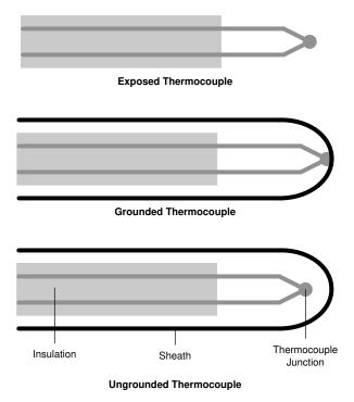
Figure 1-3. Thermocouple Construction Types
