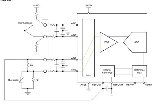
Figure 2-9. Thermocouple Measurement Circuit With Thermistor Cold-Junction Compensation
