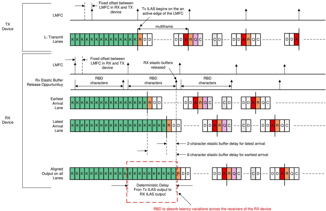
**Figure 7-1. Timing Diagram Illustrating the RX Elastic Buffer Release Opportunity in a JESD204C 8B/10B System <sup>7</sup>**
