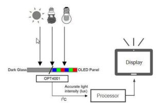
Figure 1-4. Display Brightness Diagram Using OPT4001
