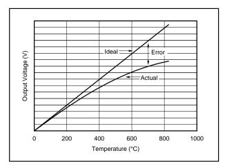
FIGURE 6. RTD Output Voltage vs Temperature.
