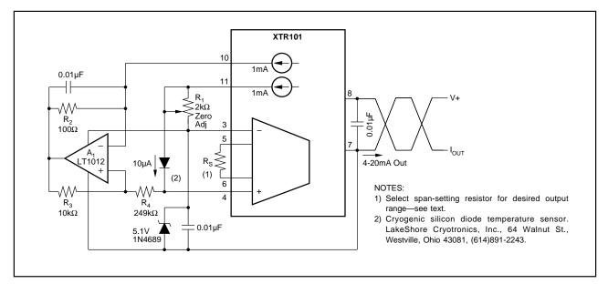
FIGURE 4. Silicon-Diode-Based Cryogenic Temperature Measurement System Using XTR101.
