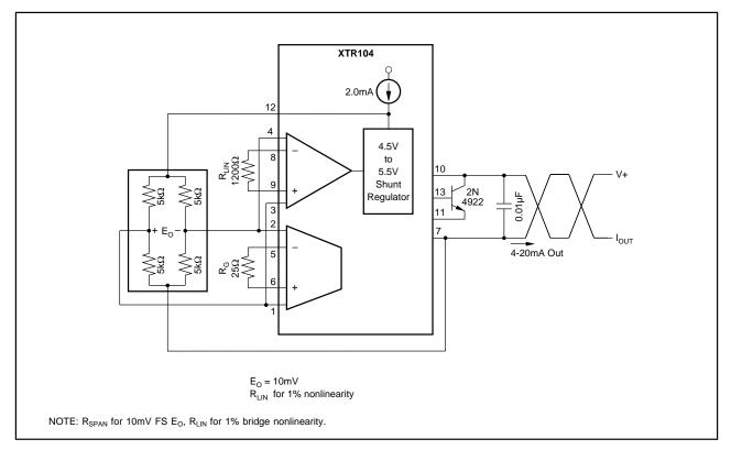
FIGURE 9. Bridge-Based Two-wire Measurement System Using XTR104.
