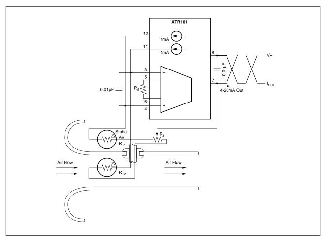
FIGURE 3C. Thermistor-Based Air Flow Rate Measurement Using XTR101.
