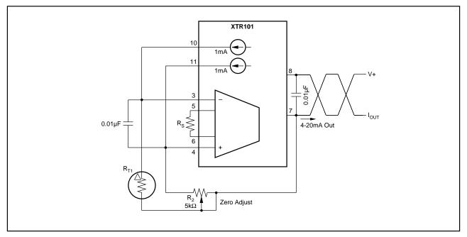
FIGURE 2. Basic Thermistor-Based Two-wire Temperature Measurement Using XTR101.
