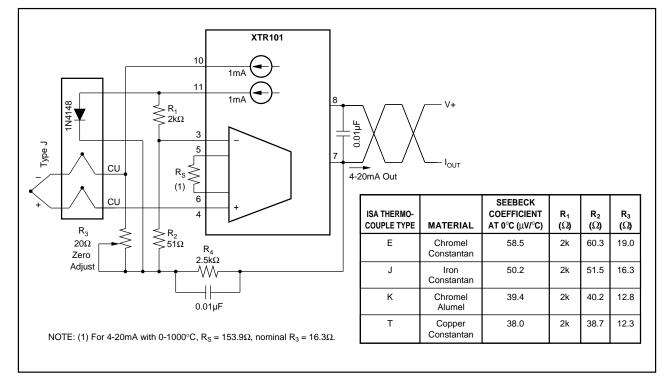
FIGURE 5. Thermocouple-Based Two-wire Temperature Measurement Using XTR101.
