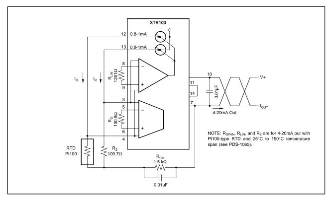
FIGURE 7. RTD-Based Two-wire Temperature Measurement Using XTR103.
