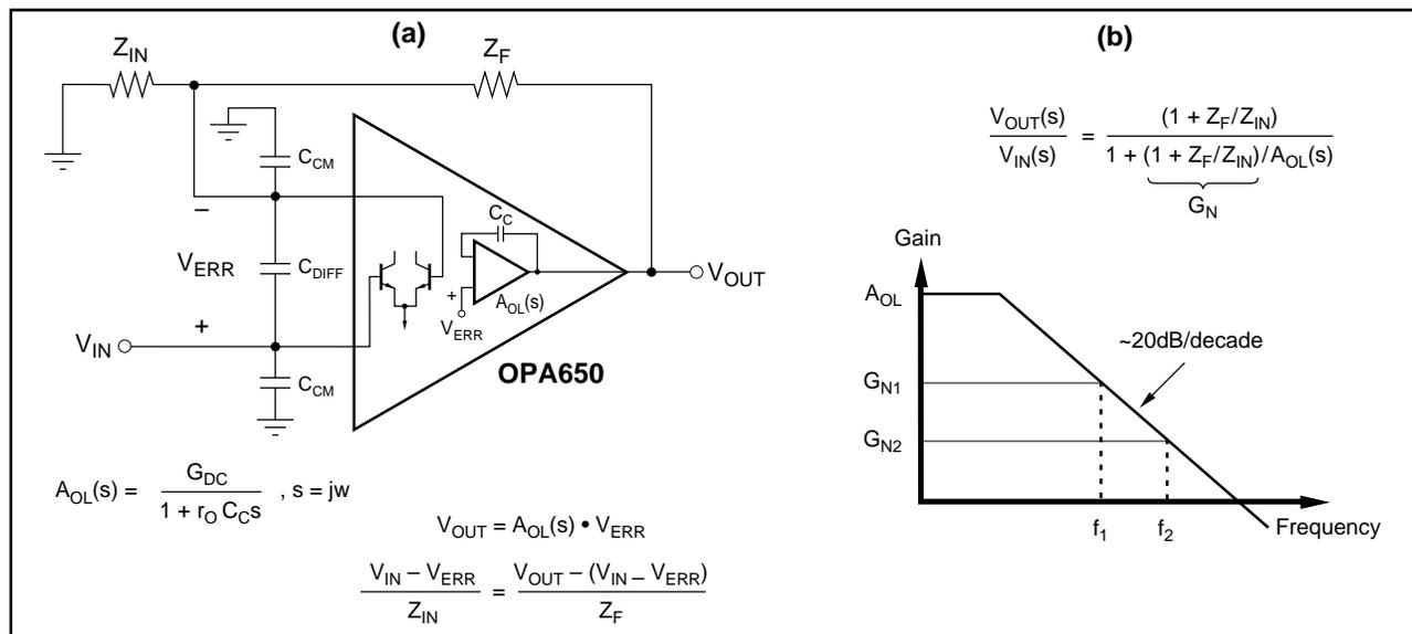
FIGURE 1a). The Model of a Voltage Feedback Amplifier Configured in a Non-Inverting Closed-Loop Configuration.
