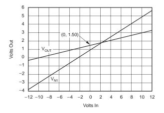
Figure 6. DC Sweep of Circuit 3
