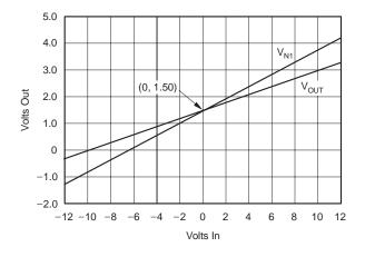
Figure 8. DC Sweep of Circuit 4
