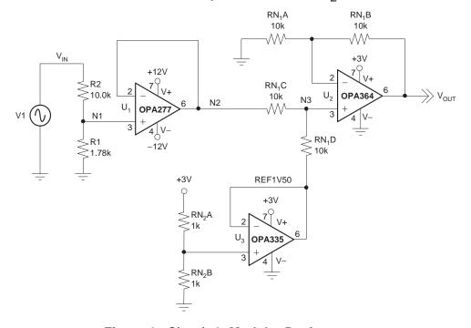
Figure 1. Circuit 1: Modular Design
