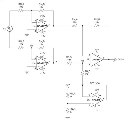
Figure 9. Circuit 5 (Circuit 1 with Differential Input)
