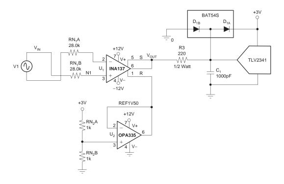
Figure 7. Circuit 4 (Circuit 3 with Differential Input)
