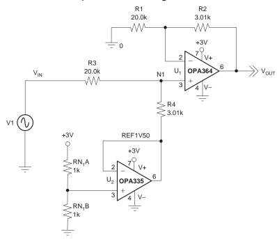
Figure 3. Circuit 2: Single-Supply/Single-Part
