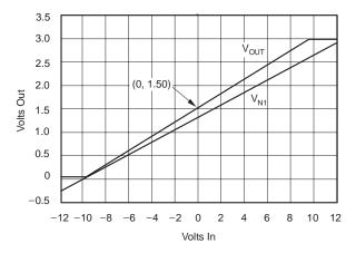
Figure 4. DC Sweep of Circuit 2
