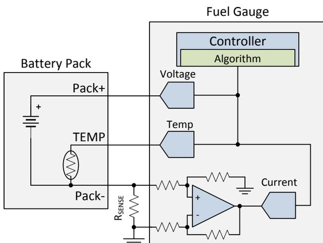
Figure 1. Battery Fuel Gauge
