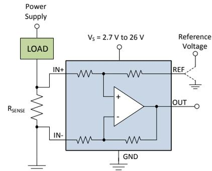
**Figure 3. INA199 Current Sense Amplifier**
