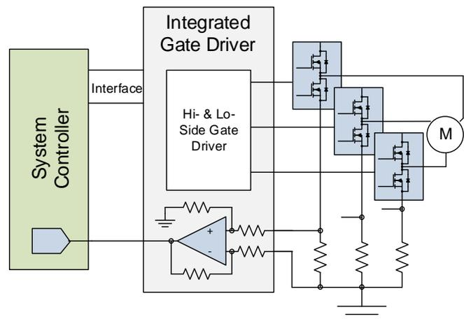
Figure 2. Gate Driver for Motor-Drive Applications
