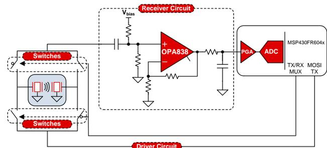
Figure 2. Typical Receive Path Circuit Using the OPA838
