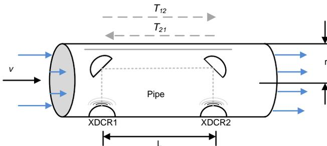
Figure 1. TOF Measurement in an Ultrasonic Flow Meter
