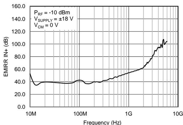
Figure 2. [OPA192](#) EMI Rejection Ratio Plot Versus Frequency
