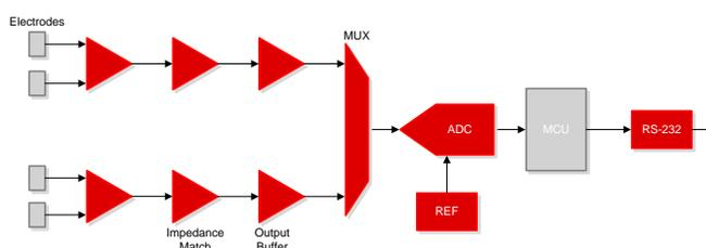
Figure 1. Typical Block Diagram for EKG
