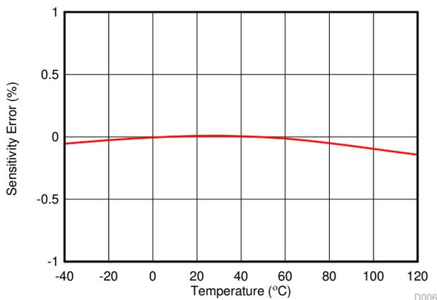
**Figure 3. TMCS1100 Typical Sensitivity Error Across Temperature**
