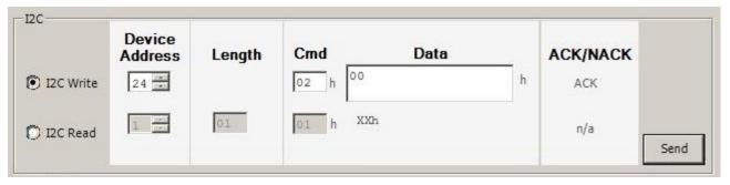
Figure 9. GUI Screen after Sending the Second Line of Initialization Code
