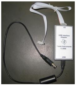
Figure 3. Picture of USB-TO-GPIO
