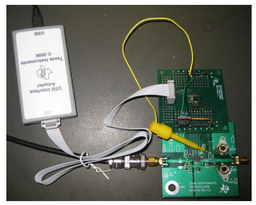
Figure 6. Total System Connection
