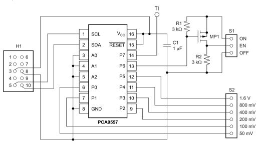
Figure 1. Schematic of I<sup>2</sup>C IO Expander Board
