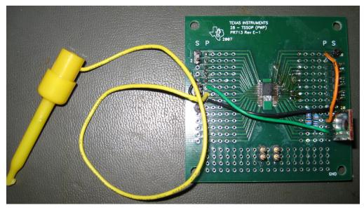
Figure 2. I<sup>2</sup>C IO Expander Board
