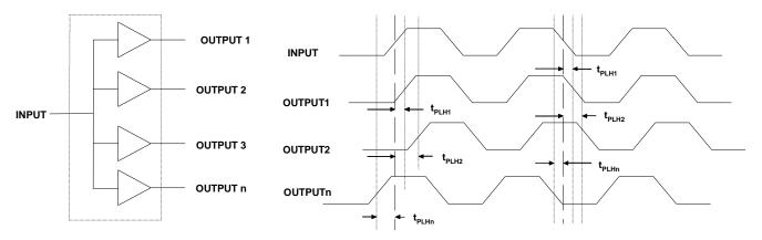
Figure 1. Output Skew (Pin-to-Pin Skew)
