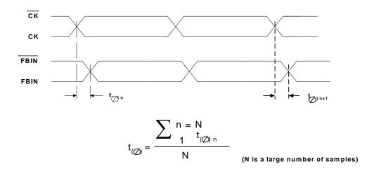
Figure 11. Static Phase Offset (Static Phase-Error)
