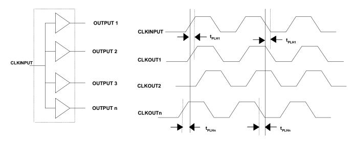
Figure 10. Propagation Delay Times, Low-to-High (tPLH) and High-to-Low (tPHL)
