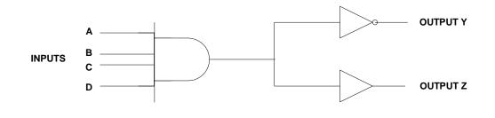
Figure 9. Example of a Gate With Input Skew
