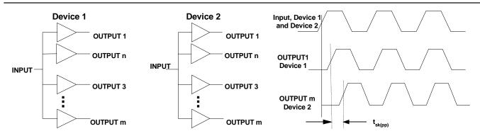
Figure 2. Part-to-Part Skew (Device-to-Device and Package Skew)
