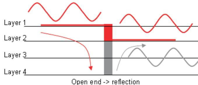
**Figure 16. Reflection Caused by Stubs in a Via**
