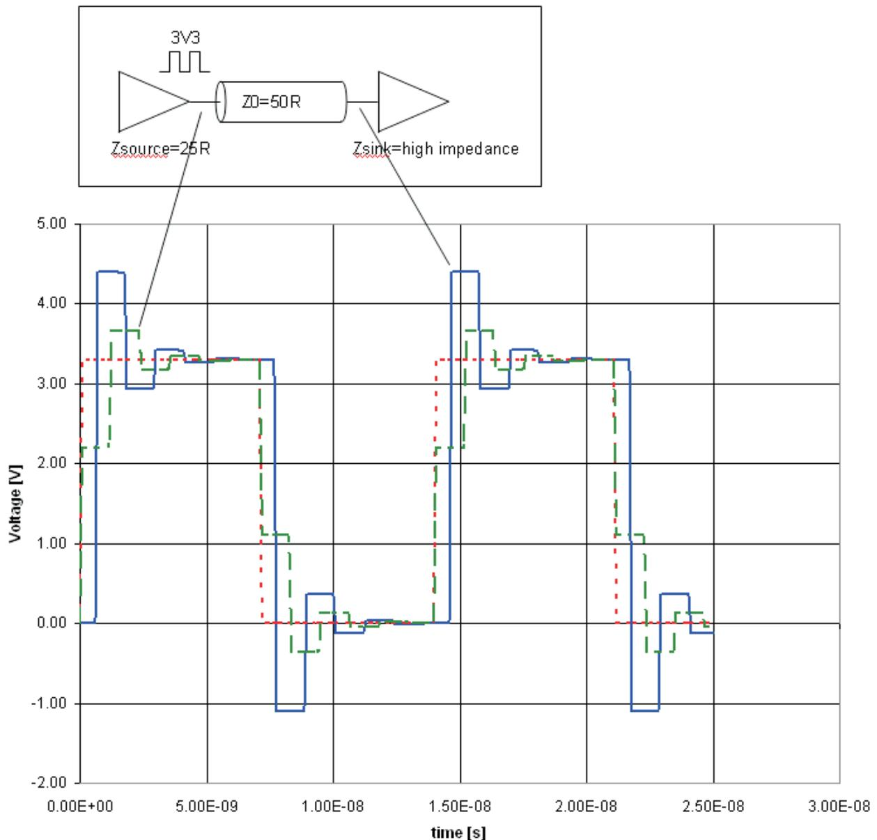
**Figure 5. Over- and Undershoots Due to Incorrect Termination**
