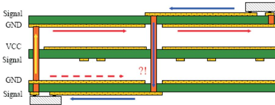
**Figure 14. Loop Areas Caused by Poor Via Placement**
