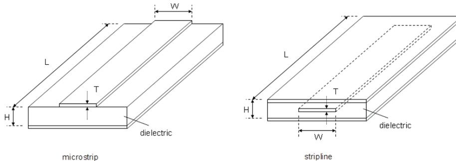
Figure 3. Structure and Dimension of Microstrip and Stripline
