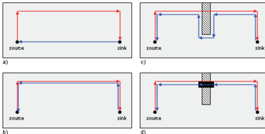
**Figure 6. Return Current and Resulting Loop Area**
