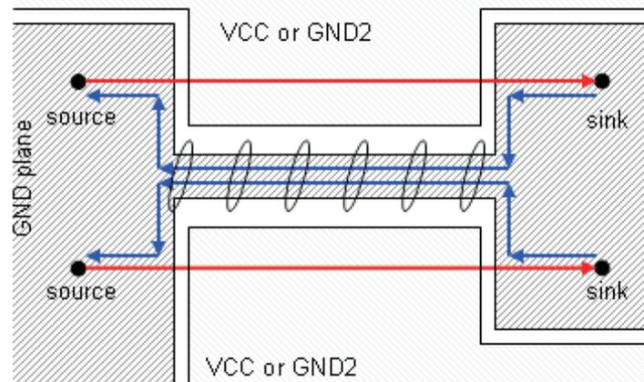
**Figure 10. Crosstalk Induced by the Return Current Path**
