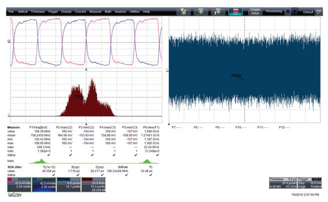
Figure 9. 156.25 MHz (6-Bit Fraction): TJ = 49.356 ps
