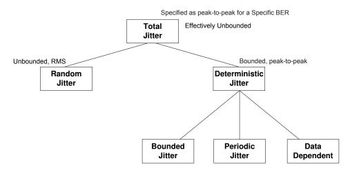
Figure 1. Total Jitter Components
