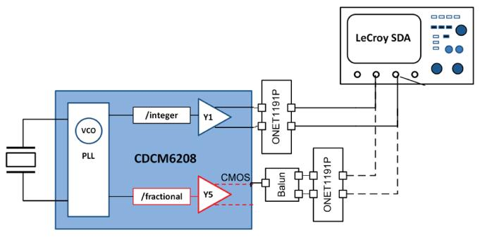
Figure 6. Improved TJ Measurement Setup With ONET1191P
