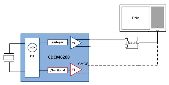
Figure 5. PNA Connection to Measure Random Jitter
