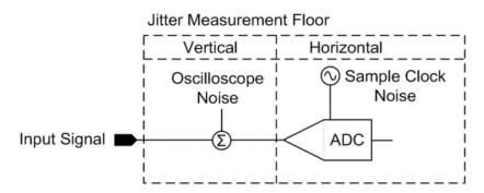
Figure 2. Oscilloscope Noise Sources
