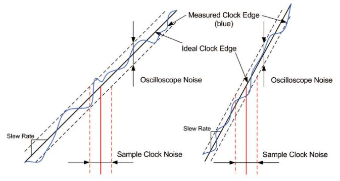
Figure 3. Slew Rate Impact on Measured Clock
