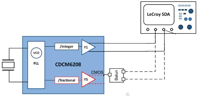
Figure 4. Traditional TJ Measurement Setup
