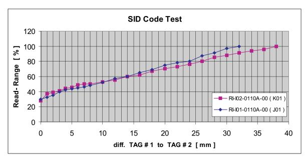
Figure 3-3. Effects of a Second Transponder Inlay
