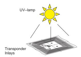
Figure 3-4. UV-Sensitivity Test Set-up
