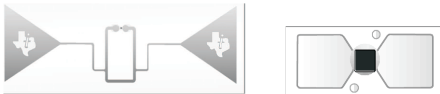
Figure 11. Ultra-High Frequency Transponder and Strap (PET Based Inlay, PET Based Device With Antenna Attachment Points)
