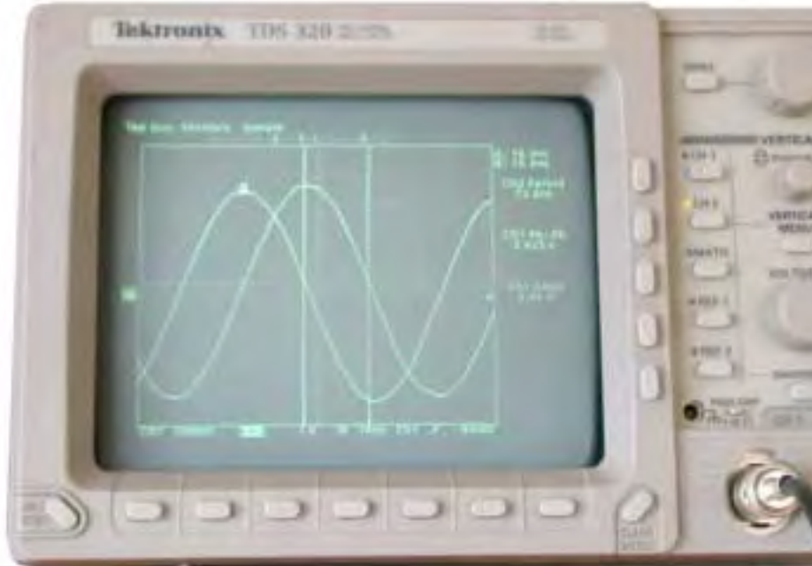
Figure 39. Scope Screen Showing the 18.4ns Offset
