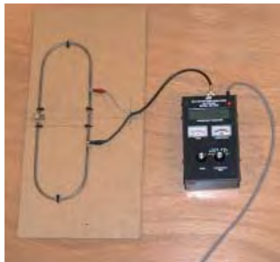
Figure 17. Using the Analyzer to Determine the Matching Points
