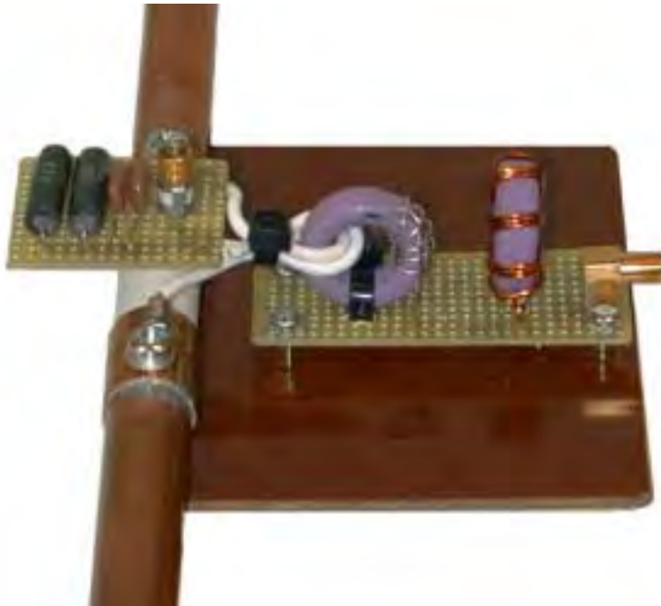
Figure 26. Transformer Circuit for Example B
