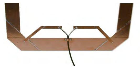
Figure 18. T-Matched Tape Antenna
