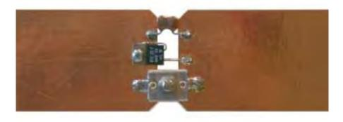
Figure 19. Resonance Adjustment and Q Damping
