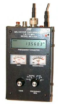
Figure 2. Antenna Analyzer
