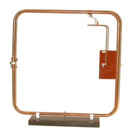
Figure 14. Gamma Matched Antenna
