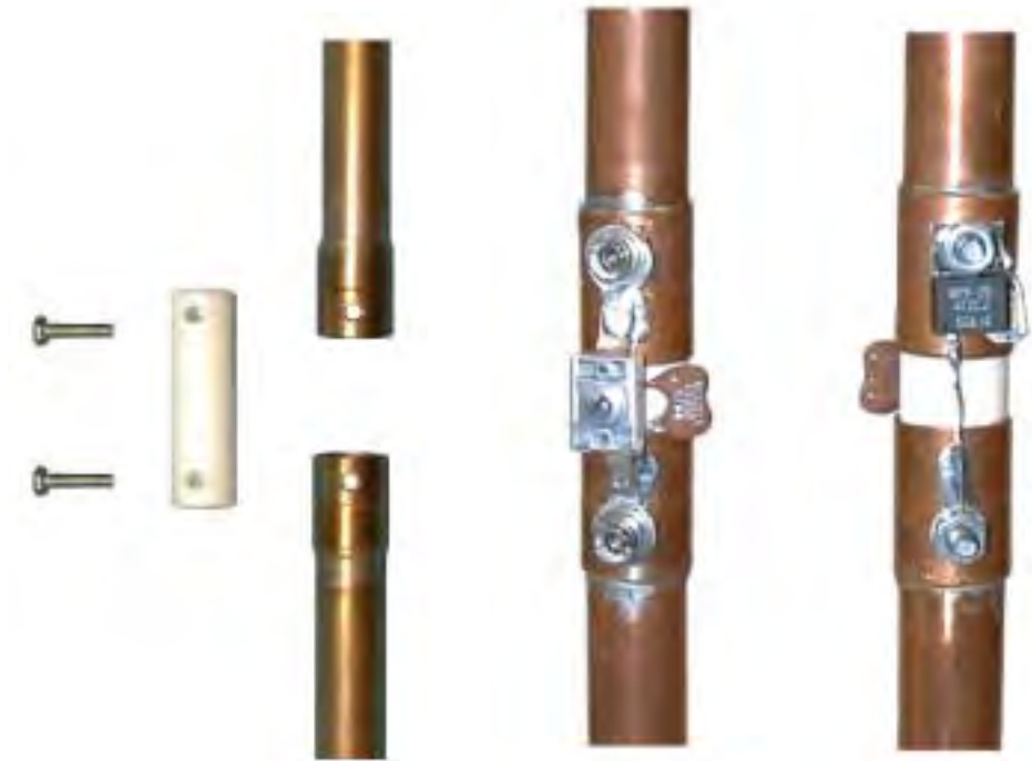
Figure 15. Joining the Loop & Attaching components
