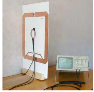
Figure 37. Both Pick-up Loops on the Basic Antenna
