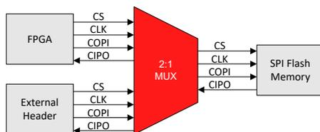
Figure 1. External Access to Flash Memory
