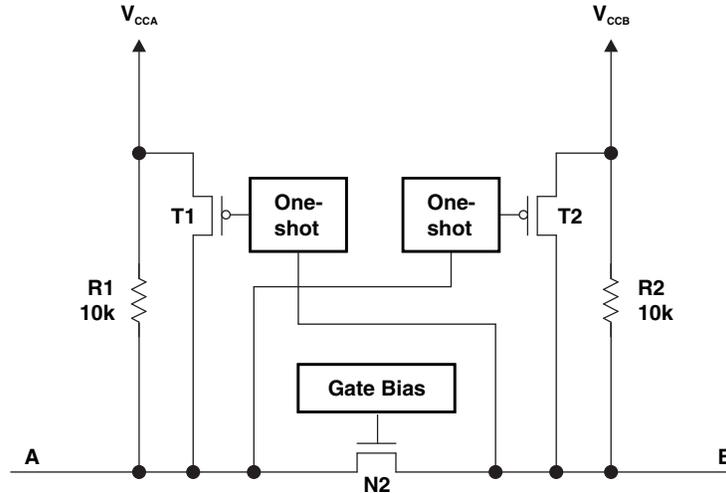
**Figure 1. Simplified TXS Architecture**
