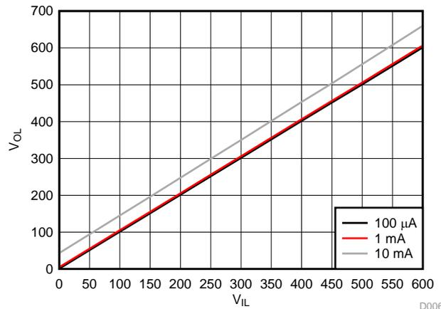
**Figure 5. LSF0108  $V_{OL}$  Versus  $V_{IL}$**
