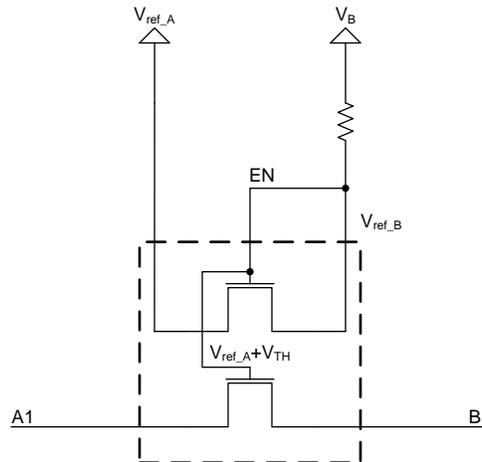
**Figure 4. LSF010x Simplified Architecture**
