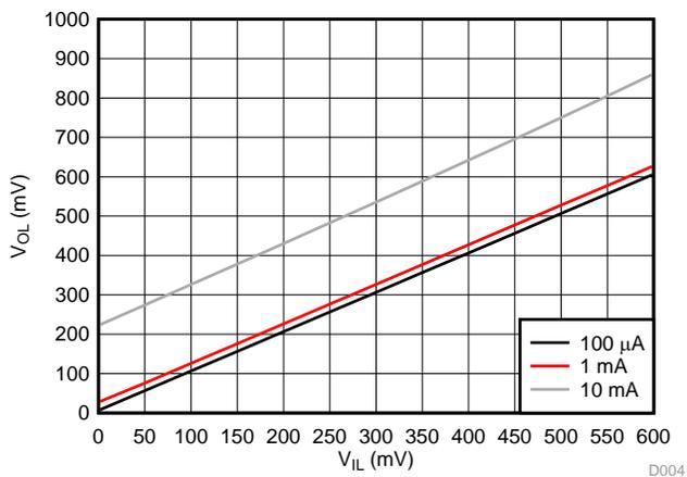
Figure 2. TXS0101  $V_{OL}$  Versus  $V_{IL}$
