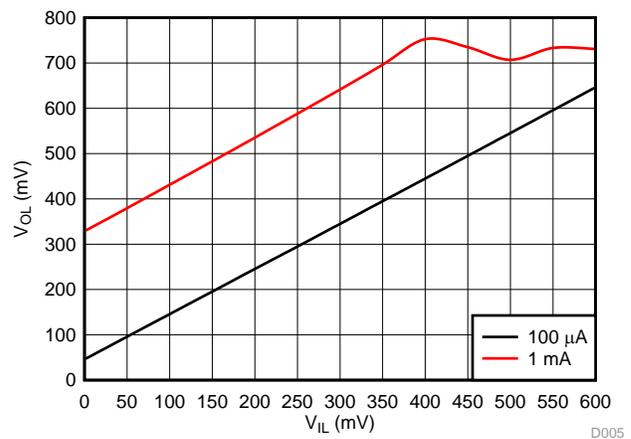
Figure 3. TXS0108E  $V_{OL}$  Versus  $V_{IL}$
