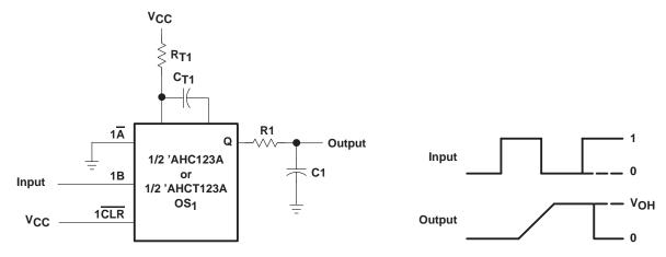
Figure 14. Frequency-Discriminator Circuit
