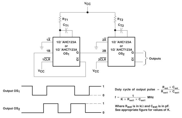
Figure 11. Low-Power Pulse Generator
