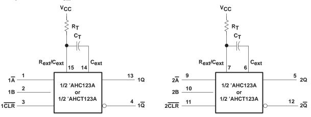
Figure 2. Timing Component Connections
