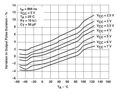
Figure 7. Variations in Output Pulse Duration for Various Temperatures and V<sub>CC</sub> Levels
