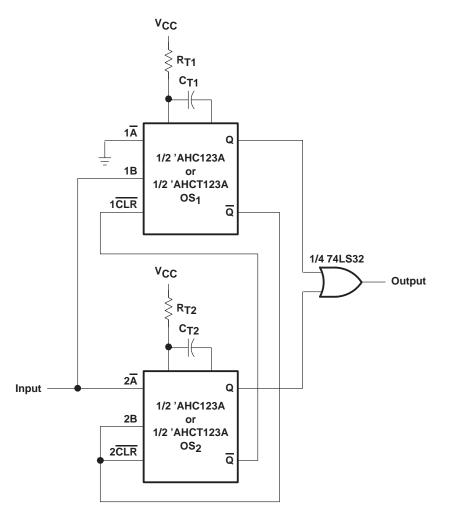
Figure 12. Negative- or Positive-Edge-Triggered One-Shot Multivibrator
