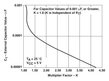
Figure 4. External Capacitance vs Multiplier Factor
