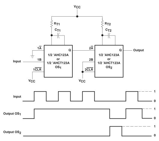
Figure 10. Missing-Pulse Detector
