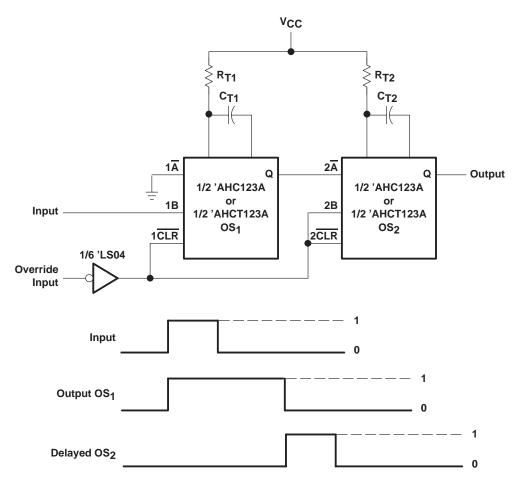
Figure 9. Delayed-Pulse Generator With Override
