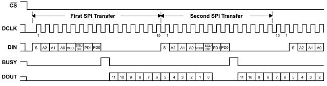
Figure 1. Typical 15-Cycle Interface
