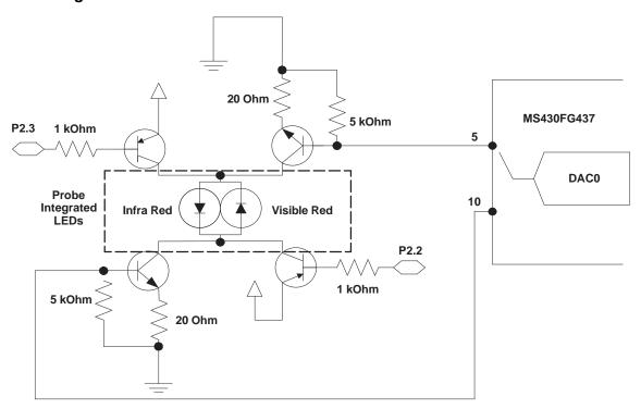
Figure 2. LED Drive Circuit
