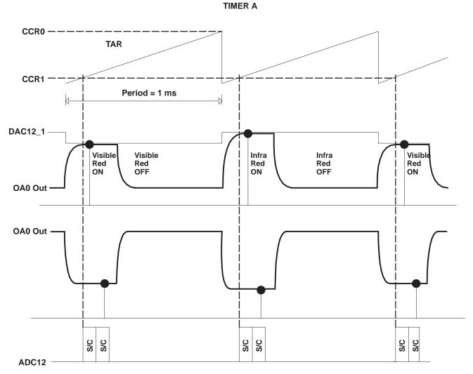
Figure 4. Time Multiplexing the Hardware
