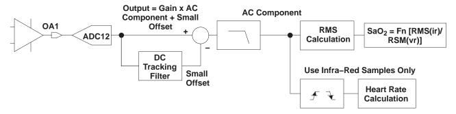
Figure 5. Signal conditioning of the AC Components
