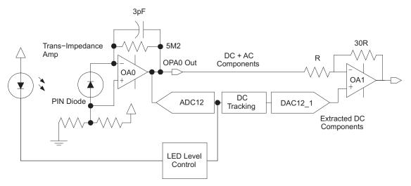
Figure 3. Input Front End Circuit and LED Control
