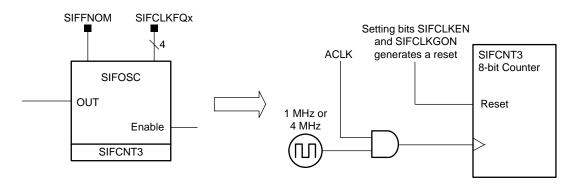
The number of ACLK cycles used for the adjustment depends on the SIFFNOM bit.
