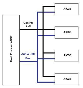
Figure 1. Four AIC33 Codecs Interfaced With a Single Host Processor/DSP
