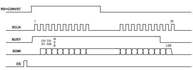
Figure 3. Timing of a Single Conversion
