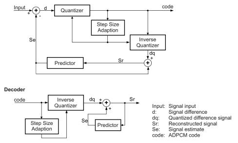
Figure 3. ADPCM Encoder and Decoder Block Diagram
