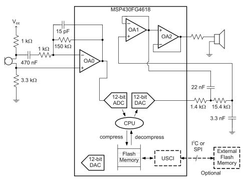
Figure 5. Signal-Chain-on-Chip Solution Using MSP430FG4618
