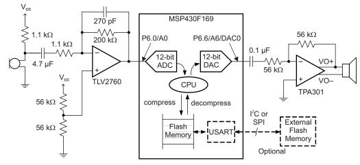
Figure 4. Signal-Chain-on-Chip Solution With MSP430F169
