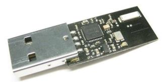
Figure 4. CC1111F32 USB RF Access Point
