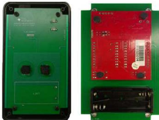
**Figure 4. Top and Bottom View of the Grip Detection BoosterPack**
