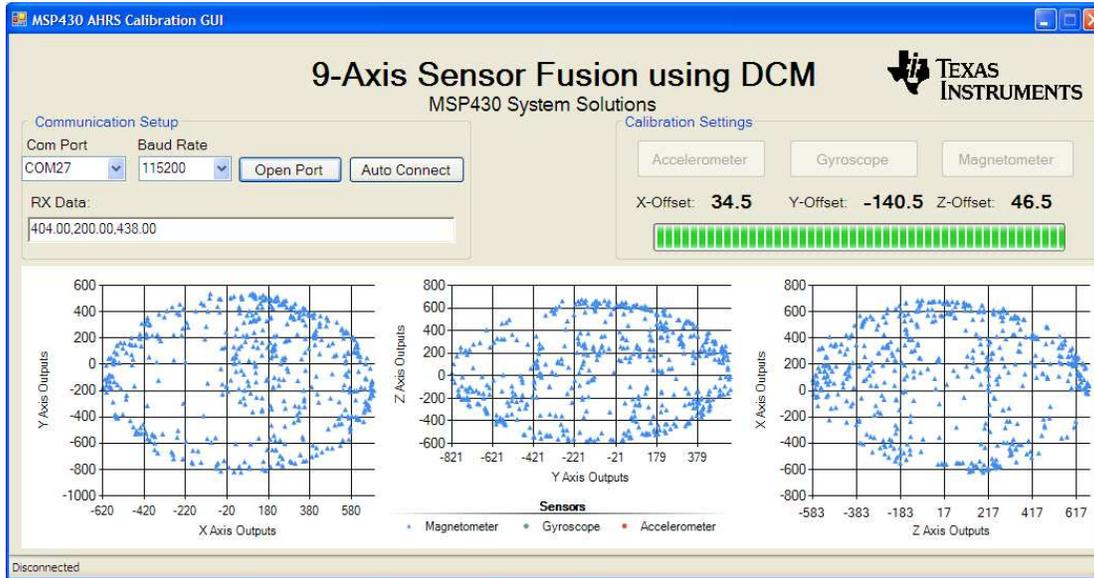
Figure 7. Magnetometer Hard Iron Calibration
