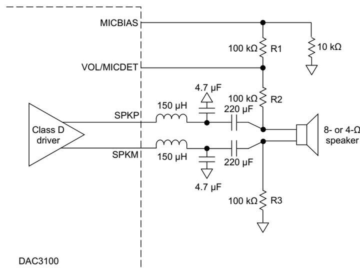
**Figure 1. Test Layout for Detection of Open Loads**
